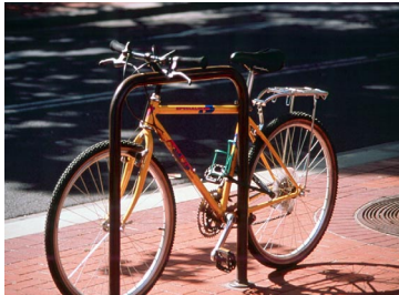
Bike racks should be located outside the walking area of the sidewalk at highly visible locations convenient to likely destinations. Racks in obscure, inconvenient, poorly lit areas are not likely to be used.
