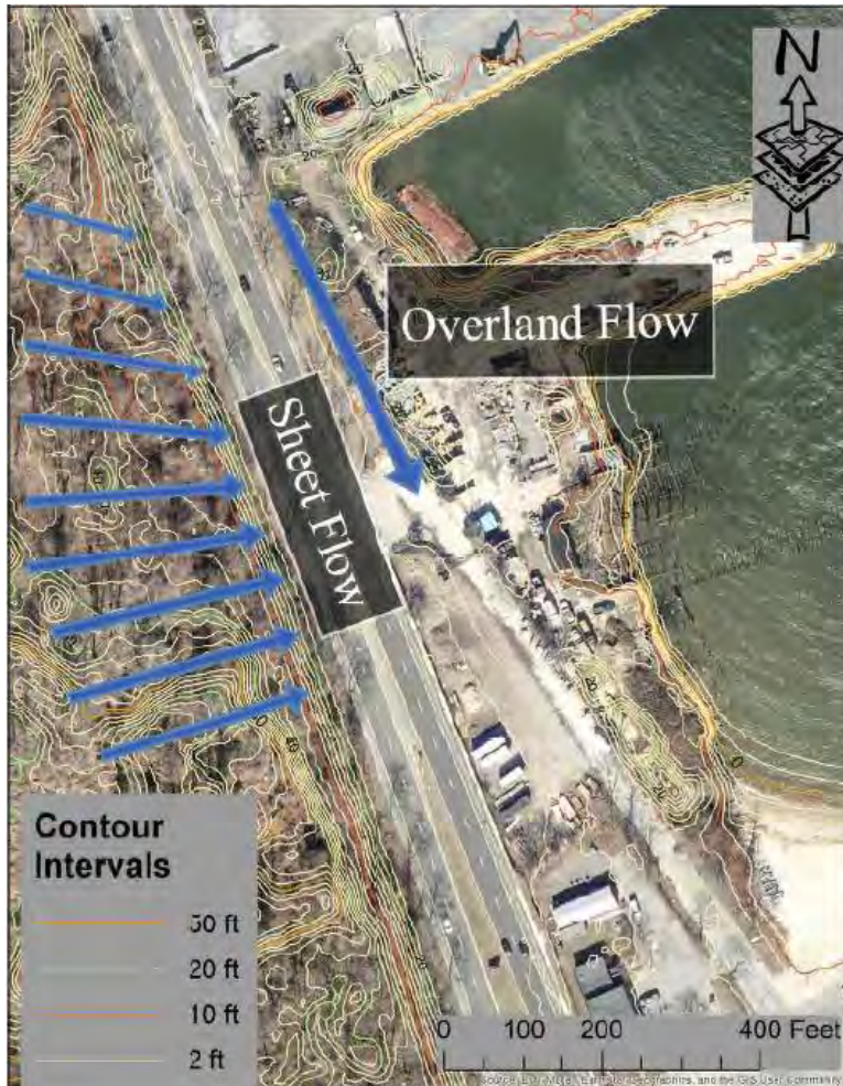
Exhibit B. A simplified map of observed patterns of stormwater entering the subject location from offsite. The site receives a large volume of overland (above-ground) flow from the Tilcon Property and the land area north of the Tilcon Property, as well as large volume of shallow subsurface flow (i.e., sheet flow) that enters the subject property under the road and from points north
