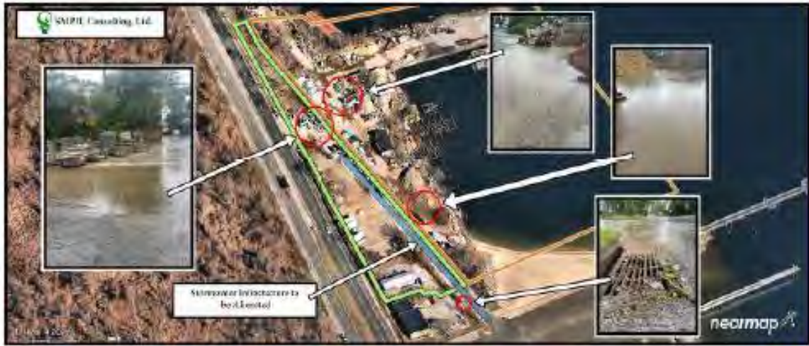
Exhibit E. A map demonstrating the location of stormwater infrastructure proposed to be alienated. Ponding of stormwater throughout the subject property due to the perched water table is also pictured.
